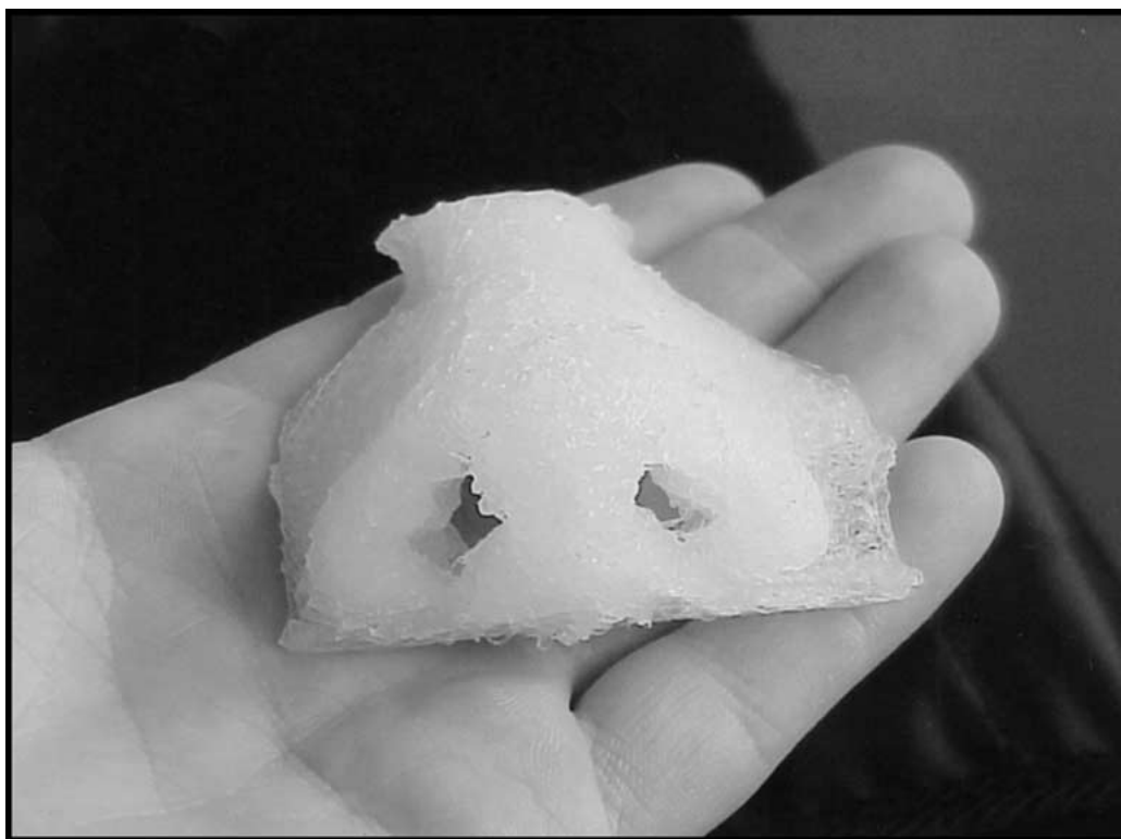
Figure 10 Silicone model of the nose prepared by 3D plotting.
